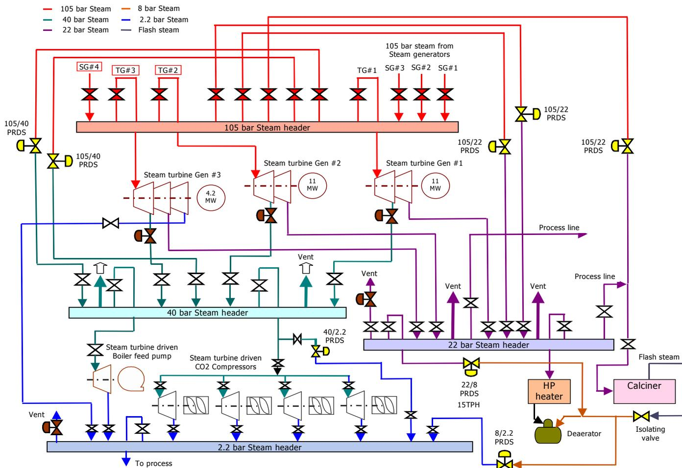
Figure 7-3: Steam Generation & Distribution System
