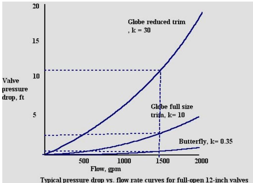
Typical pressure drop vs. flow rate curves for full-open 12-inch valves
