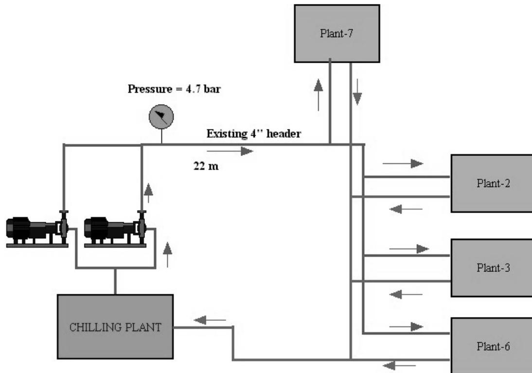
Figure 7-1: Chilled water system piping schematic
