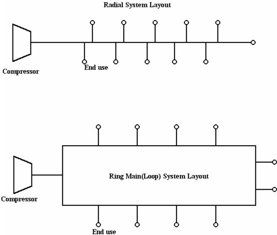
*Figure 3-2: Types o piping layout*
